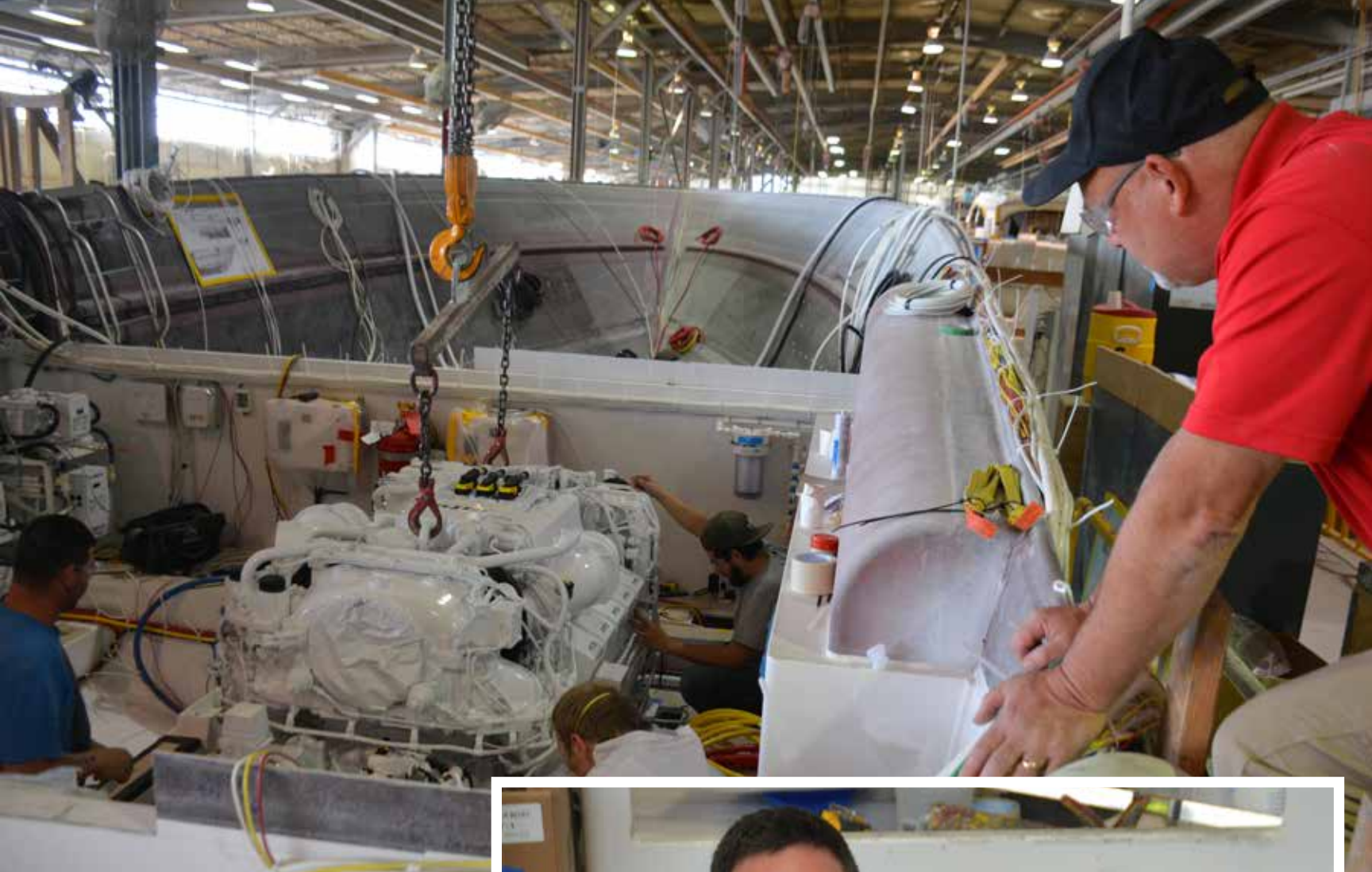
Bill Langel, Mechanical Department Foreman, oversees the placement of the first of two MTU engines in the new 58 Convertible on Line 3 in the New Grenna plant.
