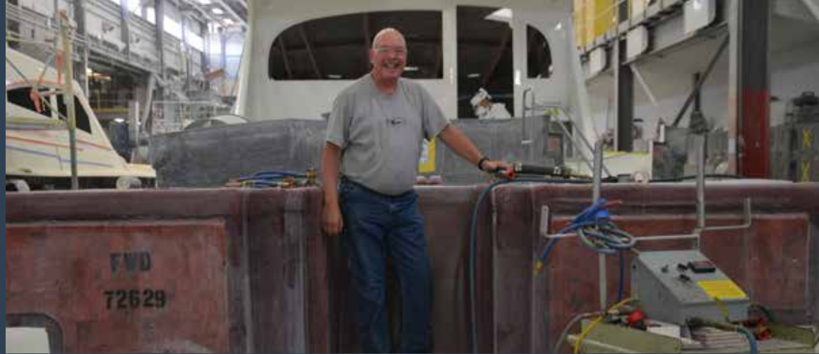
Ron Jengeleski, the “Tank Man,” stands on the fuel tank of a 72 Convertible. Ron installs the various fittings and pressure tests all of Viking’s custom-made resin-infused fuel, water and waste tanks. Total prep and testing time was about six hours for this tank.
